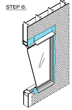
APPLY AIR-BLOC 17MR ONTO SHEATHING, LAPPING ONTO BLUESKIN SA AT WINDOW PERIMETER.
