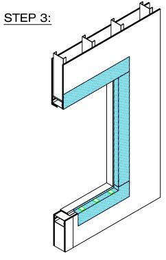
INSTALL INTERMITTENT SHIMS AT WINDOW SILL TO PROVIDE LEVEL SUPPORT AS REQUIRED BY WINDOW MANUFACTURER.
