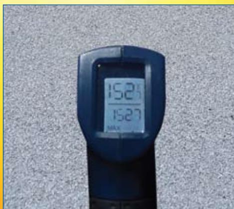
Uncoated white granulated roof = 152°F
