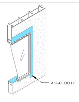
IF VOIDS OR GAPS OCCURE AT UPPER EDGE OF WINDOW HEAD FLANGE, FILL WITH AIR-BLOC LF (OR HE925 BES SEALANT) AND ALLOW TO CURE. APPLY AIR-BLOC LF LIQUID FLASHING TO WINDOW HEAD AND JAMB FLANGES TO EXTEND MINIMUM OF 2 INCHES ONTO FACE OF VERTICAL WALL AND MINIMUM OF 1 INCH ONTO WINDOW FLANGE.
