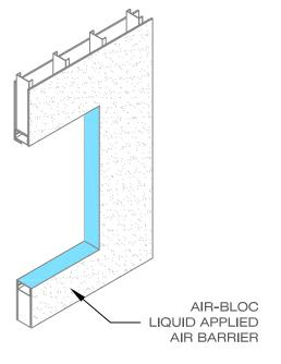
INSTALL AIR-BLOC AIR BARRIER MEMBRANE PER THE APPLICABLE HENRY AIR-BLOC TECHNICAL DATA SHEET. ALLOW AIR-BLOC MEMBRANE TO CURE PRIOR TO INSTALLATION OF WINDOW.
