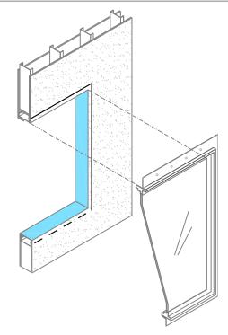
INSTALL FLANGED WINDOW AND SEALANT AS REQUIRED BY CONSTRUCTION DOCUMENTS, WINDOW MANUFACTURER OR INDUSTRY STANDARD ASTM E 2112.
