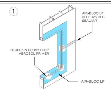
APPLY BLUESKIN SPRAY PREP AEROSOL PRIMER TO EXPOSED CUT EDGES OF GYPSUM BOARD. APPLY AIR-BLOC LF (OR HE925 BES SEALANT) TO ROUGH OPENING, JOINTS, SHEATHING SEAMS, VOIDS AND FASTENER HOLES PER THE APPLICABLE HENRY TECHNICAL DATA SHEET. EXTEND SEALANT 1" BEYOND ALL JOINTS. APPLY AIR-BLOC LF LIQUID FLASHING OVER ENTIRE ROUGH OPENING AND EXTEND ONTO FACE OF WALL 4 TO 6 INCHES.
