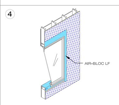
IF VOIDS OR GAPS OCCUR AT UPPER EDGE OF WINDOW HEAD FLANGE, FILL WITH AIR-BLOC LF (OR HE925 BES SEALANT) AND ALLOW TO CURE. APPLY AIR-BLOC LF LIQUID FLASHING TO WINDOW HEAD AND JAMB FLANGES TO EXTEND MINIMUM OF 2 INCHES ONTO FACE OF VERTICAL WALL AND MINIMUM OF 1 INCH ONTO WINDOW FLANGE.
