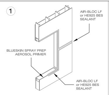
APPLY BLUESKIN SPRAY PREP AEROSOL PRIMER TO EXPOSED CUT EDGES OF GYPSUM BOARD AND ALLOW TO CURE. APPLY AIR-BLOC LF (OR HE925 BES SEALANT) TO ROUGH OPENING, JOINTS, SHEATHING SEAMS, VOIDS AND FASTENER HOLES PER THE APPLICABLE HENRY TECHNICAL DATA SHEET. EXTEND SEALANT 1" BEYOND ALL JOINTS. ALLOW TO CURE.
