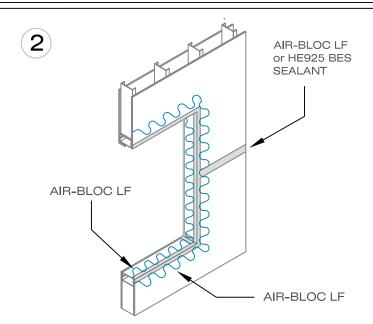
APPLY AIR-BLOC LF TO SUBSTRATE IN A SERPENTINE FASHION AROUND FACE OF WALL AND INSIDE OF ROUGH OPENING. NOTE: INSTALL SERPENTINE APPLICATION OF AIR-BLOC LF IN MANAGABLE QUANTITIES ONLY. AIR-BLOC LF MUST NOT SKIN OVER PRIOR TO TOOLING PROCEDURE DESCRIBED IN STEP 3 BELOW.
