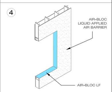
INSTALL AIR-BLOC AIR BARRIER MEMBRANE PER THE APPLICABLE HENRY TECHNICAL DATA SHEET. ALLOW AIR-BLOC MEMBRANE TO CURE PRIOR TO INSTALLATION OF WINDOW. INSTALL WINDOWS PER SPECIFICATION, WINDOW MANUFACTURER'S RECOMMENDATION OR INDUSTRY STANDARDS.
