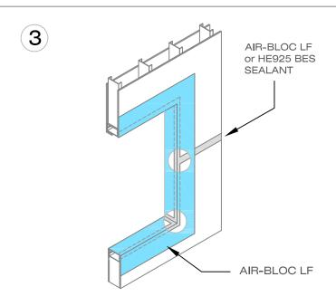
USING A TROWEL OR SPATULA, EVENLY SPREAD AIR-BLOC LF OVER ENTIRE ROUGH OPENING AND FACE OF WALL TO A DISTANCE OF 4 TO 6 INCHES. FINISHED WET FILM THICKNESS SHOULD BE AS SPECIFIED ON HENRY AIR-BLOC LF TECHNICAL DATA SHEET.
