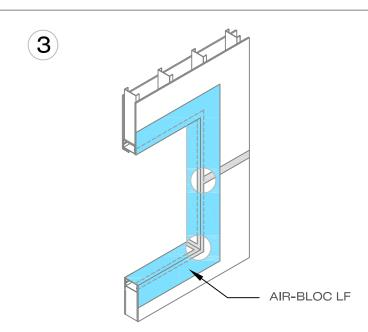
USING A TROWEL OR SPATULA, EVENLY SPREAD AIR-BLOC LF OVER ENTIRE ROUGH OPENING AND FACE OF WALL TO A DISTANCE OF 4 TO 6 INCHES. FINISHED WET FILM THICKNESS SHOULD BE AS SPECIFIED ON HENRY AIR-BLOC LF TECHNICAL DATA SHEET.
