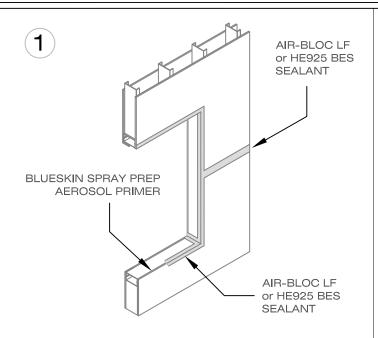
APPLY BLUESKIN SPRAY PREP AEROSOL PRIMER TO EXPOSED CUT EDGES OF GYPSUM BOARD AND ALLOW TO CURE. APPLY AIR-BLOC LF (OR HE925 BES SEALANT) TO ROUGH OPENING, JOINTS, SHEATHING SEAMS, VOIDS AND FASTENER HOLES PER THE APPLICABLE HENRY TECHNICAL DATA SHEET. EXTEND SEALANT 1" BEYOND ALL JOINTS. ALLOW TO CURE.
