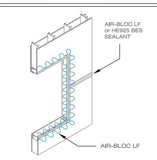
APPLY AIR-BLOC LF TO SUBSTRATE IN A SERPENTINE FASHION AROUND FACE OF WALL AND INSIDE OF ROUGH OPENING. NOTE: INSTALL SERPENTINE APPLICATION OF AIR-BLOC LF IN MANAGABLE QUANTITIES ONLY. AIR-BLOC LF MUST NOT SKIN OVER PRIOR TO TOOLING PROCEDURE DESCRIBED IN STEP 3 BELOW.
