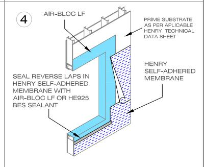
INSTALL HENRY SELF-ADHERED AIR BARRIER MEMBRANE PER THE APPLICABLE HENRY TECHNICAL DATA SHEET. SEAL REVERSE LAPS IN SELF-ADHERED MEMBRANE WITH AIR-BLOC LF OR HE925 BES SEALANT AS SHOWN. INSTALL WINDOWS PER SPECIFICATION, WINDOW MANUFACTURER'S RECOMMENDATION OR INDUSTRY STANDARDS.
