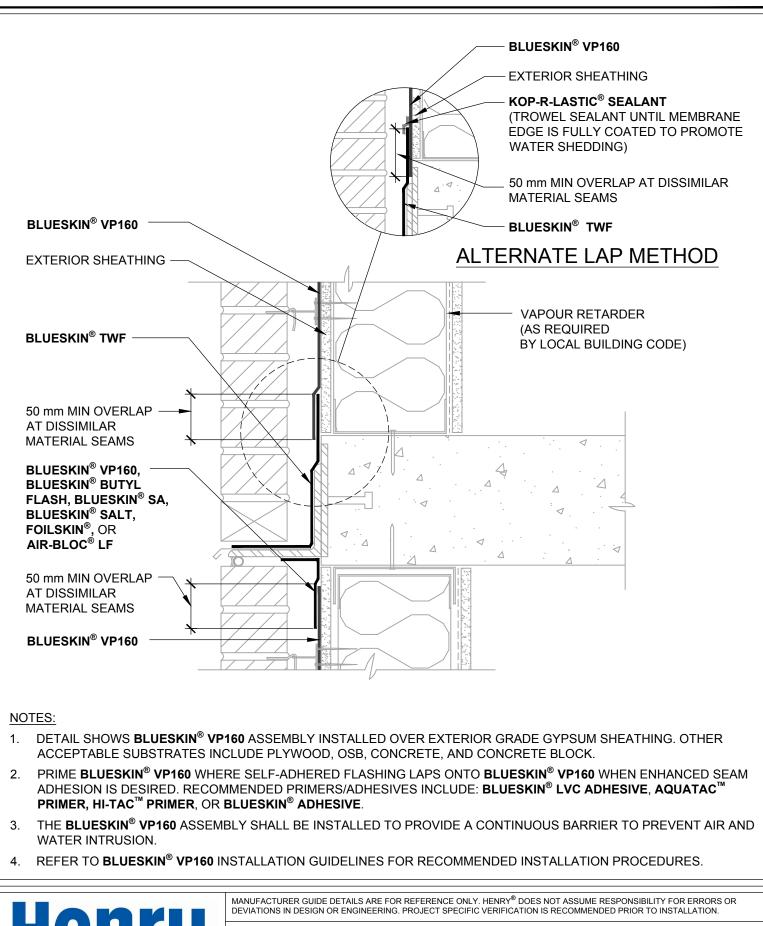
**BLUESKIN® VP160 SELF-ADHERED WATER RESISTIVE AIR BARRIER**
