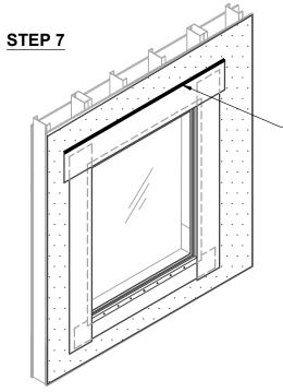
SEAL REVERSE LAP EDGES OF ROUGH OPENING FLASHINGS WITH KOP-R-LASTIC® SEALANT (TROWEL SEALANT UNTIL MEMBRANE IS FIRMLY COATED TO PROMOTE WATER SHEDDING)
