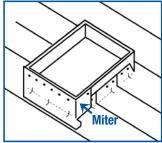
Install flashing sheet, beginning at the low end, extending 6" (150 mm) out from curb. Set in sealant. Nail at top of curb 8" (200 mm) apart on center.
