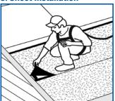
Seal at rake and set in place. Apply pressure at laps (image 14).
