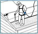
Install subsequent rows by removing the release film as well as the zip strip, then adhering the upper portion.
