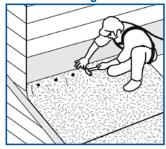
Remove lower two boards from wall to provide even substrate. Extend sheet up wall 8" (200 mm) and nail at top 12" (300 mm) apart on center.
