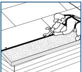
Tack nails in place along selvedge, sufficient to hold sheet temporarily. Do not drive fully as they will later be removed.
