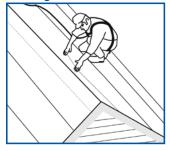
Extend ply sheets to ridge. Snap chalk line 6" (150 mm) on each side of ridge.
