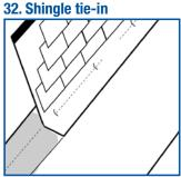
Run final ply sheet a minimum 18" (454 mm) under shingles. Set lower portion of final ply sheet into sealant as shown by shaded area.
