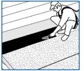
Spread sealant over surface evenly with trowel. Allow to dry for 1 hour minimum.
