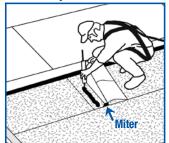
Apply rubberized sealant prior to adhering in place. Miter corner of second or middle sheet at "T" joints.
