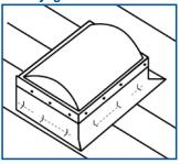
Complete flashing sheets on all sides, setting in sealant. Set skylight in place or provide metal
