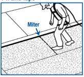
Ensure a proper seal especially at edges and overlaps by applying foot pressure...
