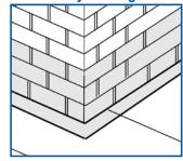
Trowel apply sealant 8" (200 mm) up chimney and 6" (150 mm) on to the roof surface. Allow to set for minimum of 1 hour.
