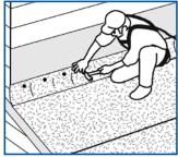
Cut flashing membrane to size. Set in sealant and nail at top 12" (300 mm) apart on center. Re-install siding after completion to cover top of flashing.
