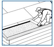
Cut rolls in half and allow to lay flat to relax for 20 minutes. Align at eave.
