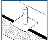
Stop application of sheet at soil pipe. Place pre-formed flashing over soil pipe.
