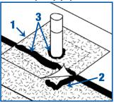
1. Cut piece 4" (100 mm) larger than flashing. 2. Set in sealant spread 3" (76 mm) wide around perimeter. 3. Apply sealant over granulated flashing at lap line and around pipe.
