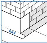
Install flashing sheet "A". Extend 8" (200 mm) up chimney and 6" (150 mm) on to roof surface.
