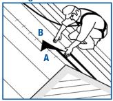
Run ply sheet "A" over ridge 6' (150 mm). Run ply sheet from other side of roof "B" over ridge a minimum of 6" (150 mm). Set in sealant where sheet overlaps granules.
