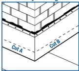
Install flashing sheets "B", "C" and "D". Install termination bar at top of flashing sheet and apply bead of sealant.
