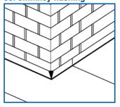
Run ply sheets a minimum of 2" (50 mm) up chimney.
