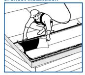
Remove release film from lower portion and set in place. Be careful to ensure that sheet lays flat and wrinkle free.
