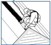
Apply sealant along chalked line. Cut strips of sheet and set into sealant. Note: Roof slope not shown to scale.
