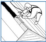
Continue installing ridge flashing sheets overlapping 3" (76 mm) and nailing through 3" (76 mm) selvedge.
