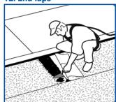
Spread sealant over granulated area to be overlapped.
