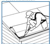
Fold back lower portion of sheet and apply rubberized sealant to metal edge and rake.
