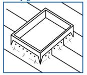
Turn ply sheets up at curb a minimum of 2" (50 mm) and nail 8" (200 mm) apart on center.
